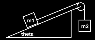
Two masses are connected by a light string as shown in the figure. The incline and peg are smooth. Find the acceleration of the masses and the tension in the string for theta = 30 degrees and m1 = m2 = 5kg.
