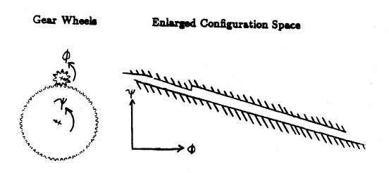
Figure 4.2: Gear wheels and corresponding configuration space
