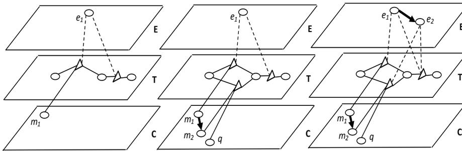
**Figure 3: A tiered network. Nodes in the explanation layer (E) represent explanations composed of well-founded TMS support. The TMS layer (T) contains TMS nodes (circles) and justifications (triangles) that support physical behaviors. The conceptual knowledge layer (C) consists of processes and quantities. Left: before a model revision; Middle: after revising  $m_1$  as  $m_2$  using new quantity  $q$  (see Figure 1) Right: after computing a preference for  $e_2$  over  $e_1$ .**
