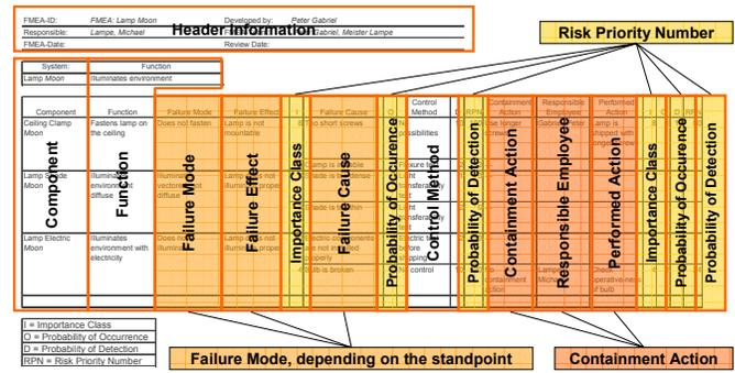
Figure 1: Identification of elements of an FMEA
