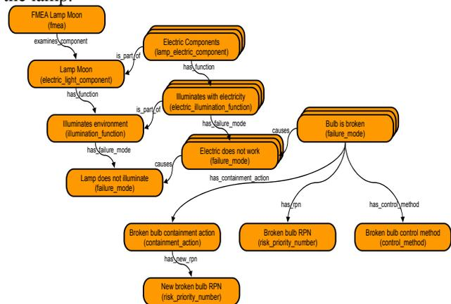
Figure 4: Instances of an ontology-based FMEA
