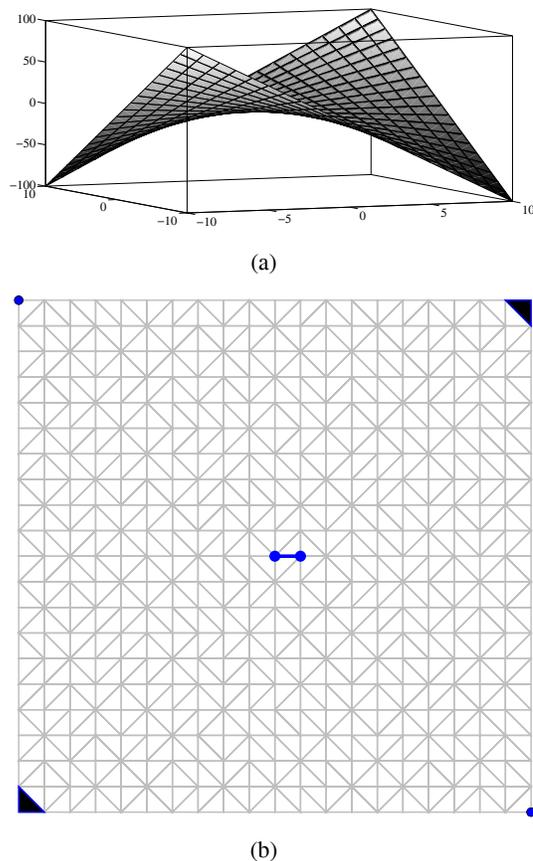
Figure 1: Function  $f(x, y) = xy$  and the triangulation of its domain with two minima (circles), two maxima (triangles) and a saddle in the middle.
