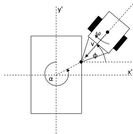
Figure 3: Variables defining the position and orientation of the robot relative to the block.
