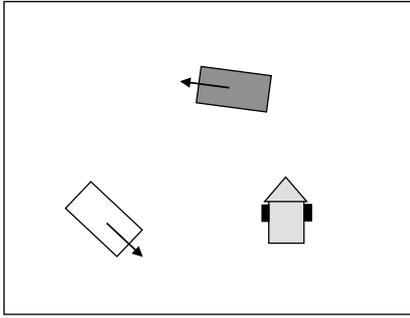
Figure 1: The robot's task is to move the object (dark rectangle) to the goal position (white rectangle) with the block in the indicated orientation (arrows). The robot may push the object by the tip of its triangular bumper. Dark rectangles of the robot's shape are the robot's wheels.
