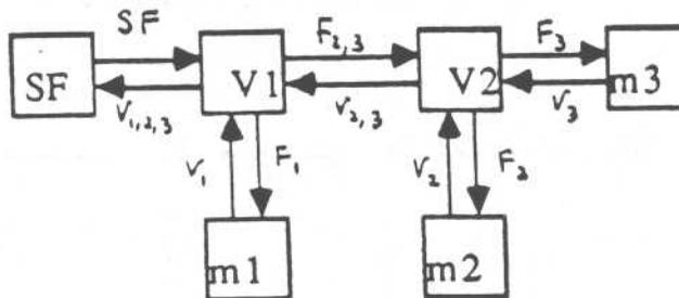
Figure 7: The force and velocity flow directions for the three-block example
