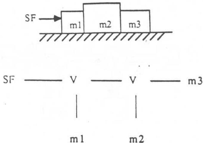
Figure 6: 1) A Series of blocks 2) Blocks in bond graph
