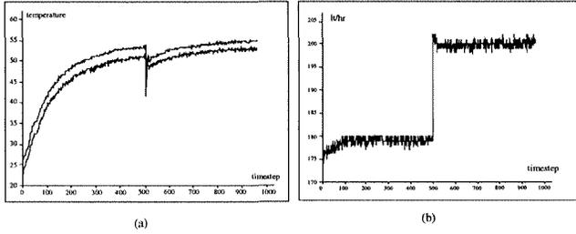
Figure 5: (a) Temperature data with one to two pumps running; (b) Flow changes with one to two pumps running.
