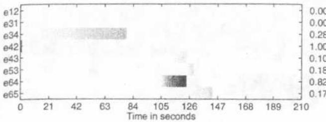
Fig. 5: Graphical representation of the statistical properties of the tank system for fault  $f_1$  and initial event  $e_{42}$
