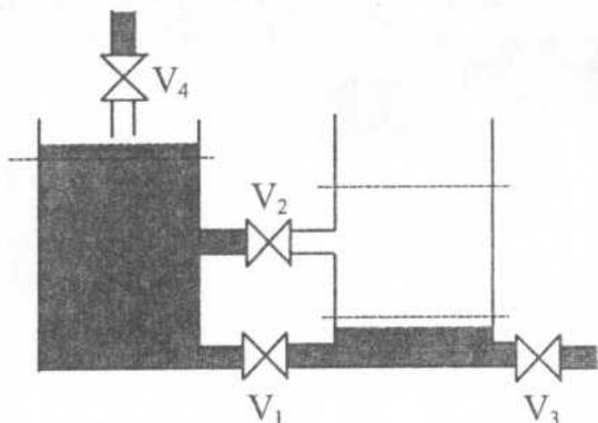
Fig. 2: Example of a batch process
