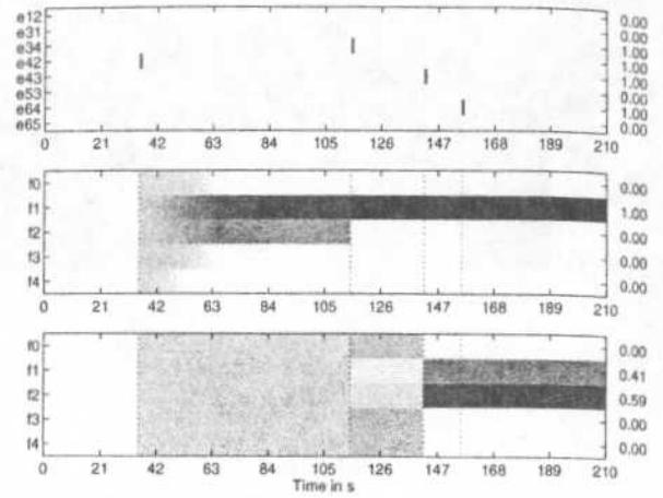
Fig. 10: Fault diagnosis for fault  $f_1$  with  $e_{42}$  being the initial event
