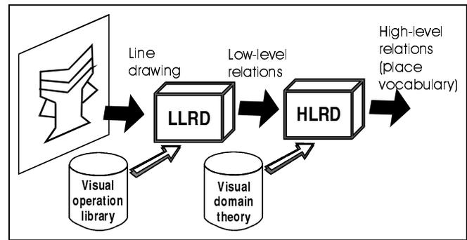
**Figure 2: A simplified schematic of GeoRep's architecture.**
