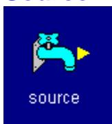
Sources start streams. There are two types of streams: those that are part of loops and those that start at sources and end at sinks. Using splitters and mixers, it is possible to combine the two types of streams, but for every source, there must be a sink and vice-versa.
