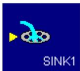
Sinks end streams. There are two types of streams: those that are part of loops and those that start at sources and end at sinks. Using splitters and mixers, it is possible to combine the two types of streams, but for every sink, there must be a source and vice-versa.
