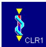
Coolers cool the working fluid flowing through them by allowing heat to flow to the environment. This process may cause the fluid to change phase.
