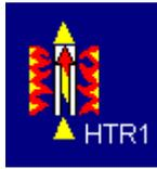
Heaters add thermal energy to the working fluid flowing through them. This may cause the fluid to change phase. A heater may be used to represent a boiler, a superheater, a reheater, a combustion chamber, or a nuclear reactor.
