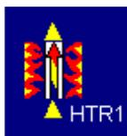
The two yellow triangles are the heater's *ports*. They indicate the direction of flow through the heater (in this case, bottom to top), and they enable you to connect the heater to other components.
