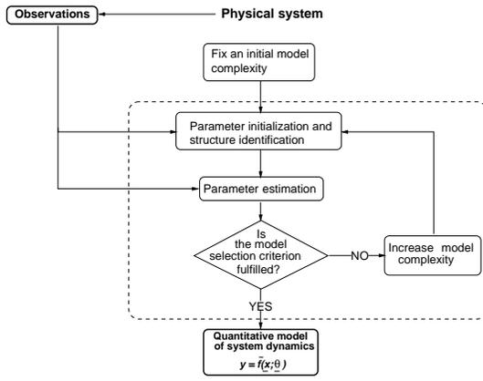
Figure 1: Main steps in data-driven approaches
