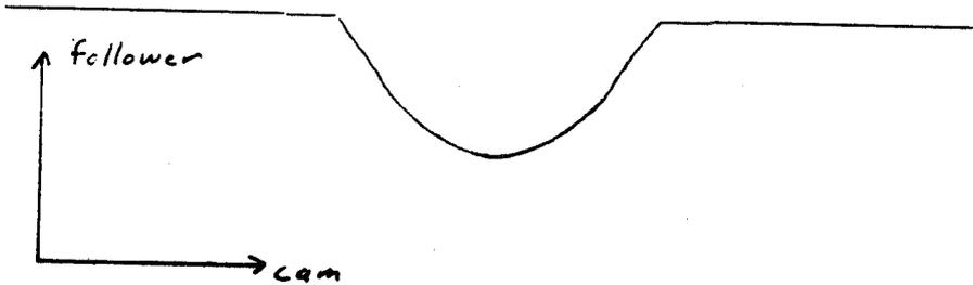
Figure 9.34: Configuration Space for Cam
