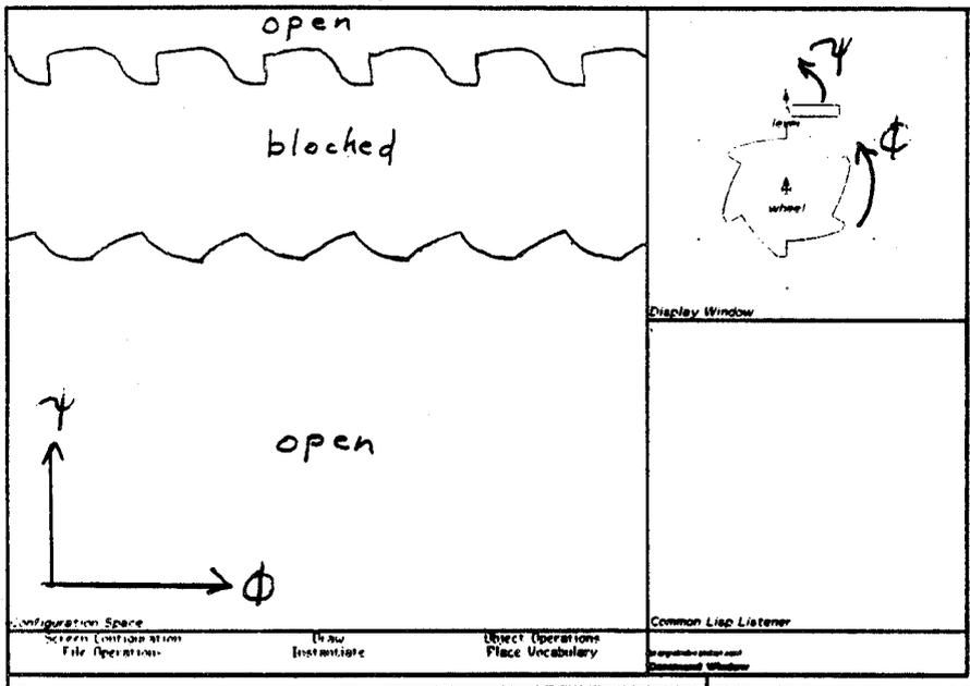
Figure 9.9: The configuration space for ratchet and pawl
