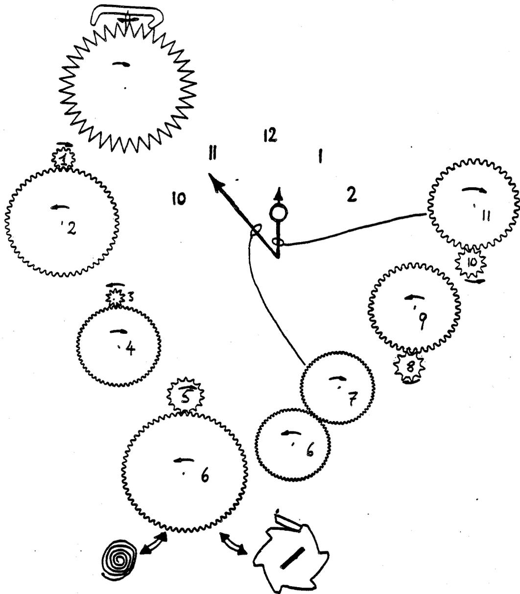
Figure 9.1: Two dimensional representation of the QRG clock
