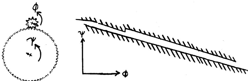
Figure 4.2: Gear wheels and corresponding configuration space
