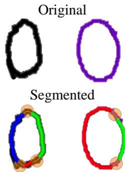
Figure 3. Error segmenting an ellipse with improved edge-segmentation.
