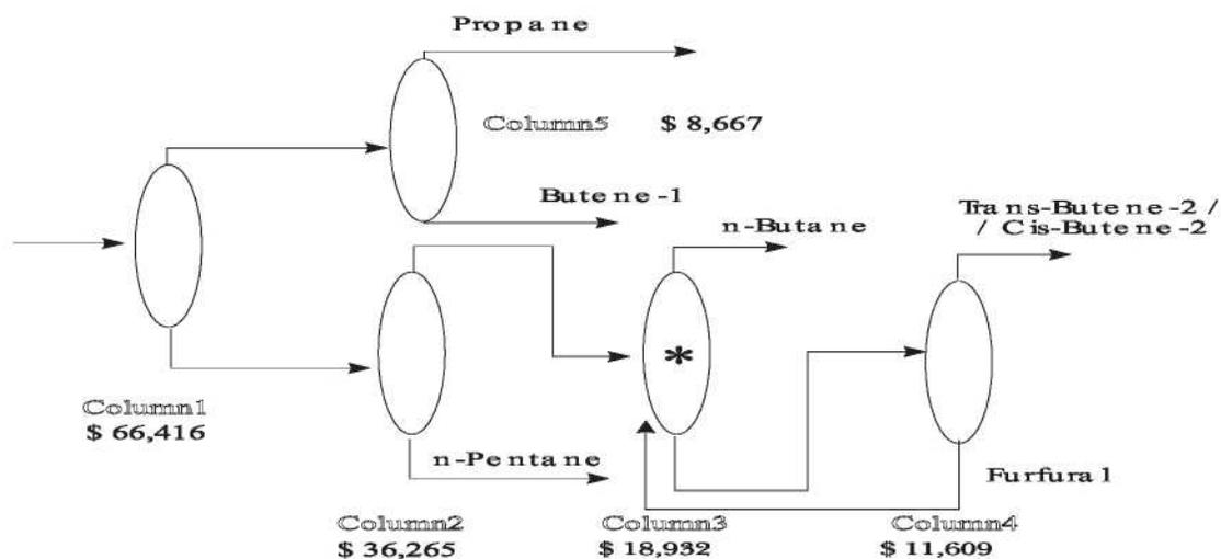
**Figure 1.1:** Problem specification and possible design for the n-Butylene purification problem. Columns with an asterisk (\*) correspond to extractive distillation units. The rest are ordinary distillation columns.
