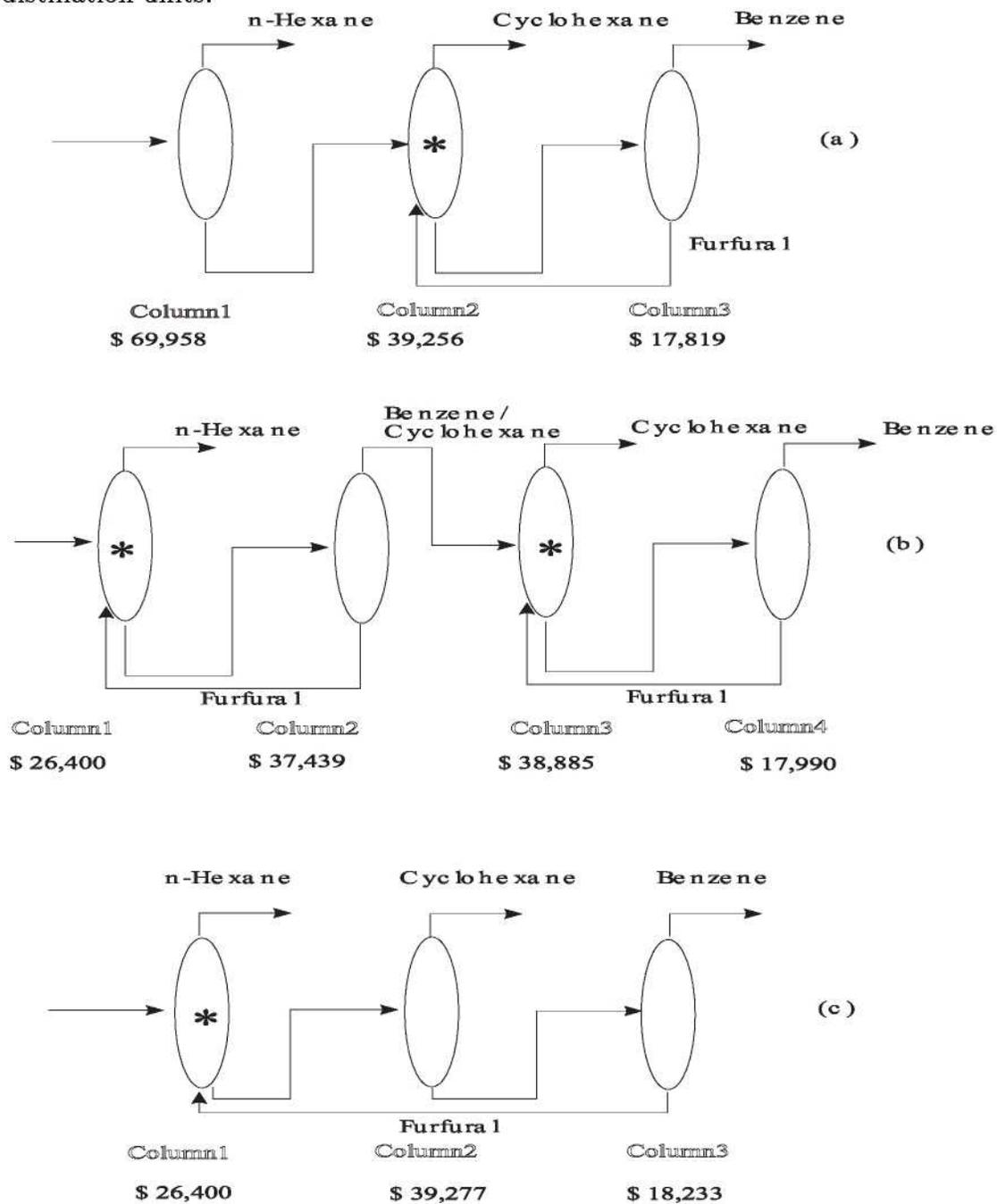
**Figure 6.7:** The flowsheets generated by the Seader & Westerberg method for the  $C_6$  separation problem. The columns with an asterisk (\*) indicate extractive distillation units.
