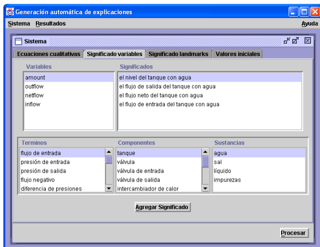
Figure 1. Semantic information associated with each state variable. Each variable (e.g., amount highlighted in the upper half) has information about its meaning ( the amount of water in the tank ), and information about the substance and related component (e.g., input flow highlighted in the lower half, is associated with a particular tank and with water )
