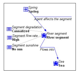
Figure 3: The simplest scenario for a river in our simulation tool composed of a spring, a river segment, and the sea. The river segment here is specified as canalized, high flow rate and no sunshine reaching the river.
