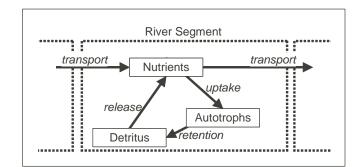
Figure 1: The implemented components of the nutrient spiraling concept, with nutrients as the only component moving downstream (*spiraling*).
