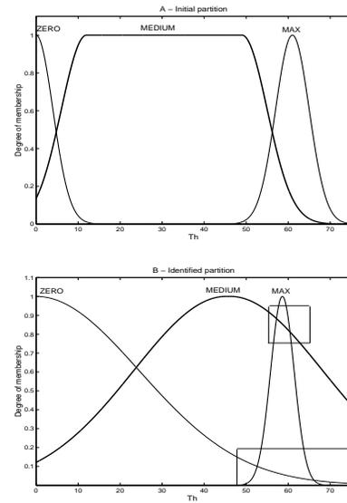
Figure 8: Gaussian/double-gaussian  $\mu$ 's: A - Initial; B - Identified.
