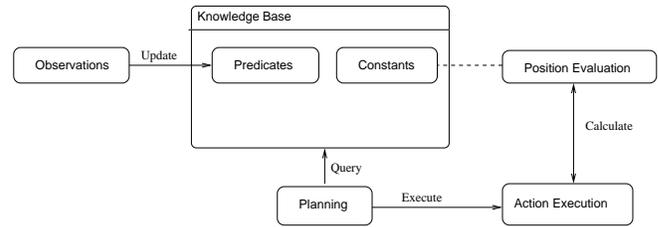
Figure 4: Abstracting numerical data to symbolic data, performing qualitative reasoning on this symbolic data, and grounding the resulting actions to create numerical motion commands.
