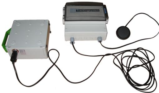
Figure 2: The implemented prototype of the container tracking unit.
