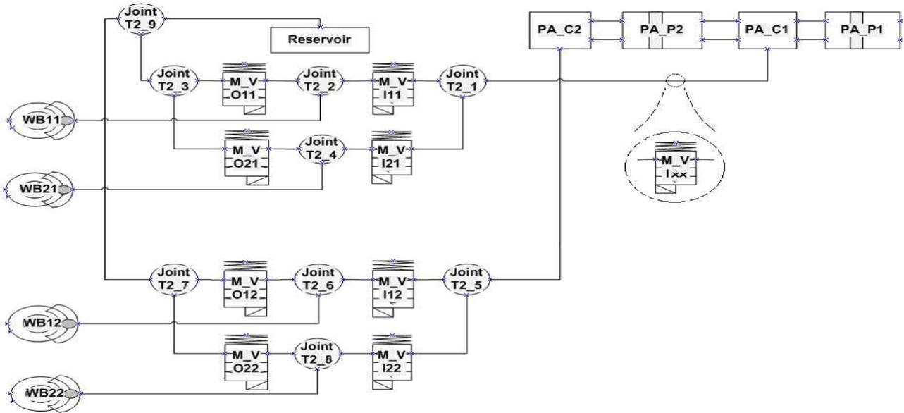
Figure 2 - Braking system. Pressure is generated by two pistons, PA\_P1,2, in two chambers, PA\_CA1,2, and reaches the wheel brakes, WB<sub>ij</sub>, via open inlet valves, M\_VI<sub>ij</sub>, while outflow is blocked by closed outlet valves, M\_VO<sub>ij</sub>. The impact of inserting another valve, M\_Vixx, is discussed in section 5.3
