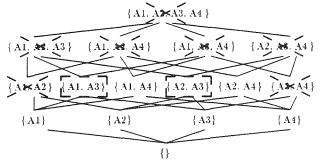
First, note that at the bottom the lattice is rooted in the original model — since there are no assumptions no exaggeration has been performed. And as we move upwards through the lattice the models become simpler, since each assumption makes an additional term insignificant, which then drops out of the equations.
