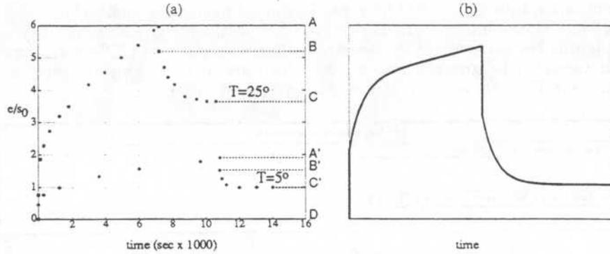
Figure 6 - Experimental creep plots (a) and their qualitative abstraction (b): experimental values of  $\epsilon(t)/s_0$  are plotted against time at two different temperature levels.
