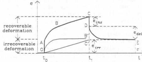
Figure 4 - A typical strain response to a creep test.
