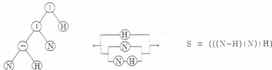
Figure 2 - Different representations of the same rheological structure: rooted binary tree, series-parallel circuit, rheological formula.
