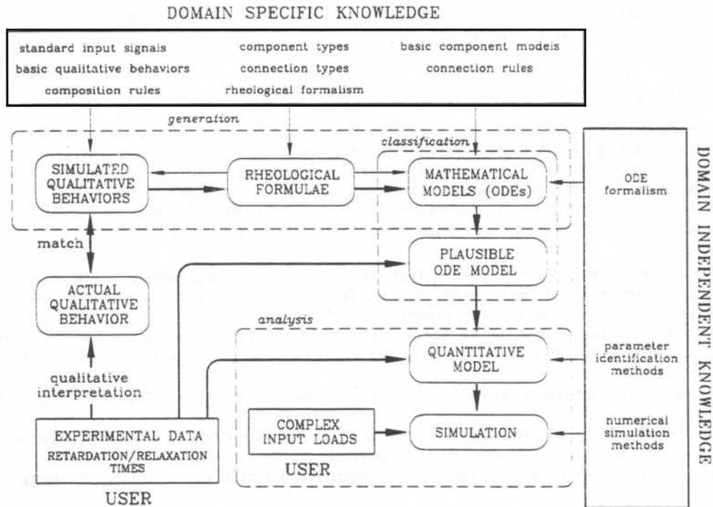
Figure 1 - Overview of the system. The main tasks of library generation, material classification and analysis are outlined by pointing out the basic steps they consist of. Arrows basically denote control flow: more precisely, thick arrows track data flows while marginal thin arrows denote system interactions with specific pieces of knowledge.
