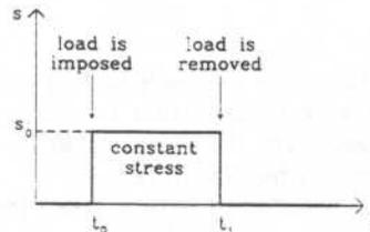
Figure 3 - Creep test: a constant stress state is imposed for a time  $\Delta t = t_1 - t_0$ .
