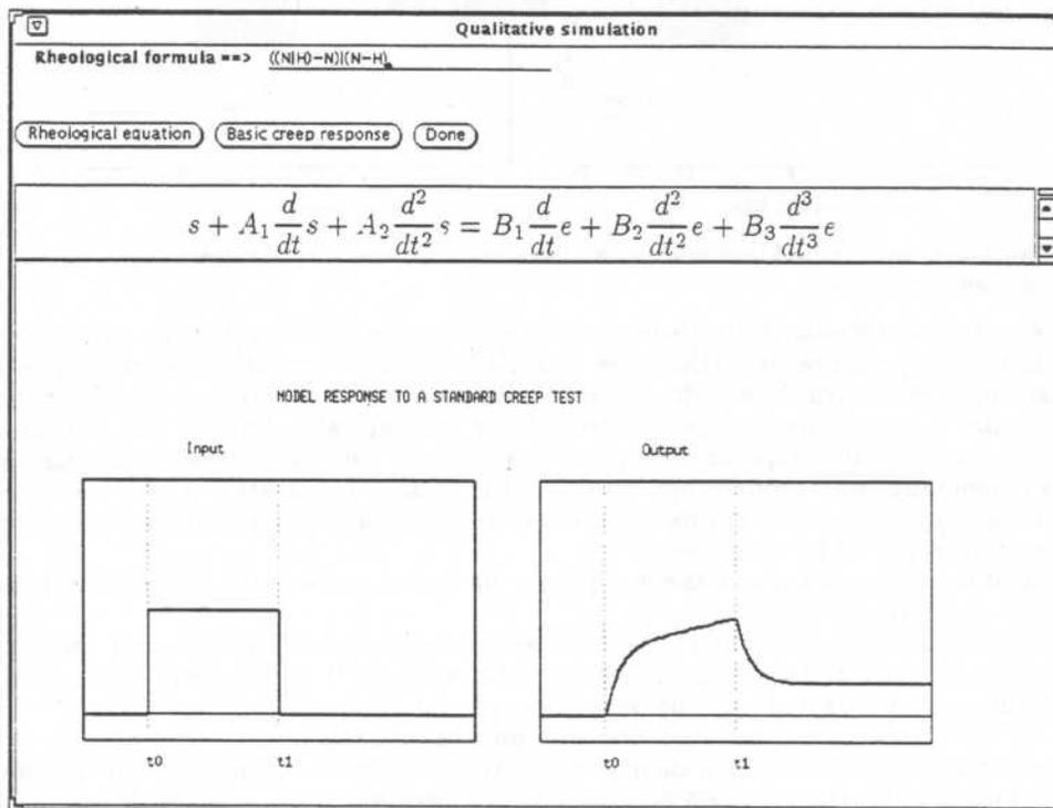
Figure 5 - Outcome of the computer simulation of the behaviour of the material modelled by the formula  $((N|H) - N)|(N - H)$  in response to a creep test in simple tension.
