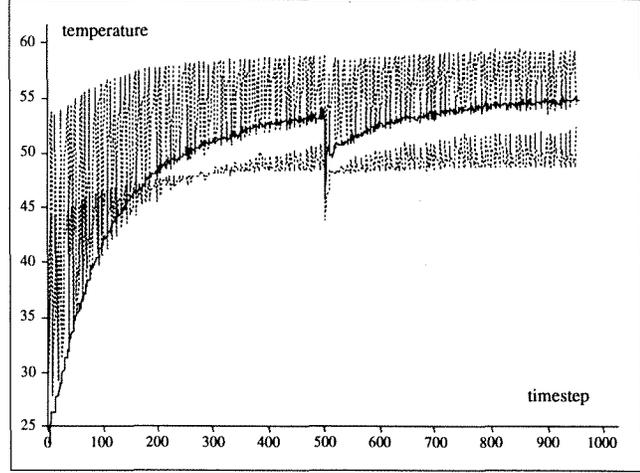
Figure 7: Dotted lines: boiler output temperature prediction ranges; solid line: real measurements. Interpolation time step  $n = 10$ .
