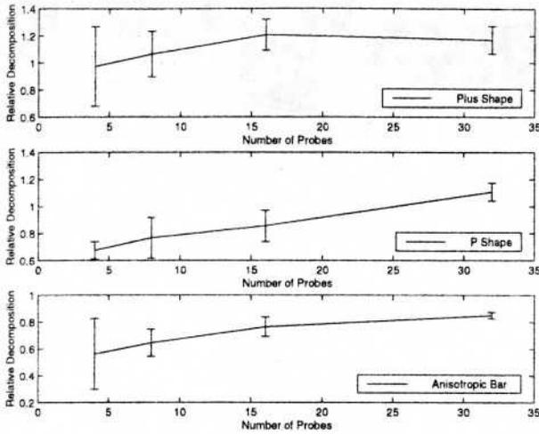
Figure 11: Performance data indicate that the probe clustering algorithm supports trading decomposition quality for computation. Results are relative to spectral partitioning.
