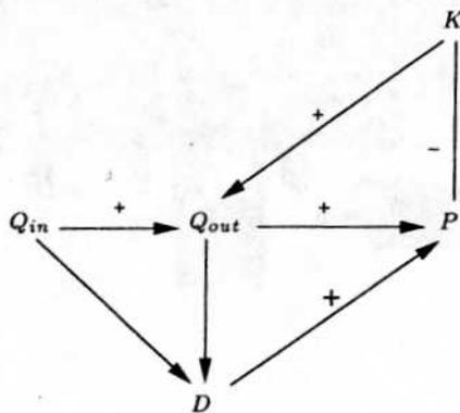
Figure 3: Causal graph with signs for the bathtub
