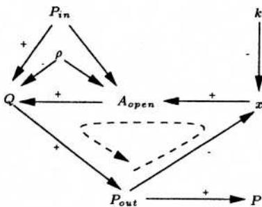
Figure 6: Causal graph with signs for the pressure regulator
