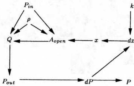
Figure 5: Causal graph for the pressure regulator
